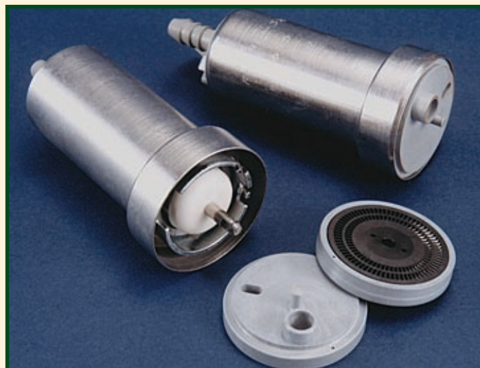
The DCSS pump's 50mm-enlarged section houses a 44mm impeller with an outer and an inner pumping channel to improve pumping efficiency by 50% over a single-channel turbine pump
