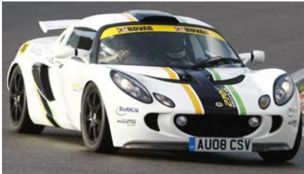
Lotus Exige tri-fuel can run on any mixture of petrol, bio-ethanol or methanol
